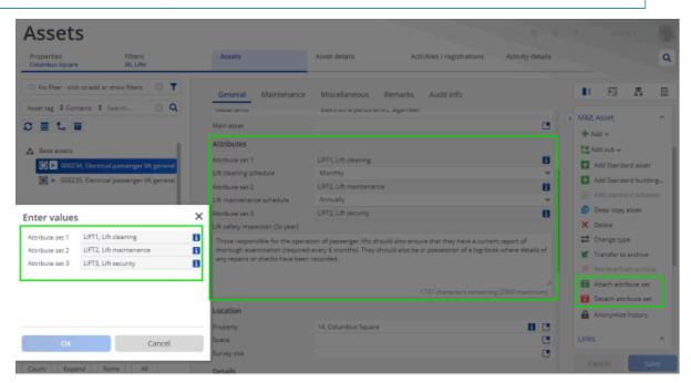
After linking an attribute set, the characteristics specified in the attribute definition are displayed on the elements panel. In this example two drop-down type attribute sets and one multiline type are attached.
